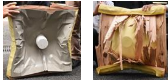
Fig. 2 Effect of reinforcement with aramid fiber A roof reinforced with the advanced fiber absorbed the impact when a fist-sized cinder crashed into it
